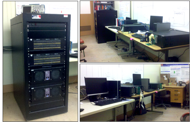
Fig. 3. Real Time HIL System for Simulation of Power Systems.
