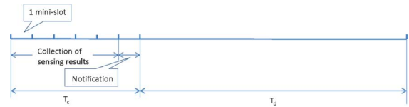
Fig. 2. Control slot T_c and data slot T_d .
