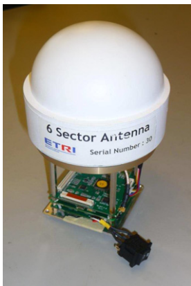
(c) Hardware Platform With Sectored Antenna
