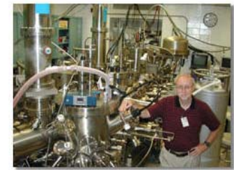
Dr. Phillip E. Thompson of the Naval Research Laboratory next to his molecular beam epitaxy system. Credit: Phillip E. Thompson, Naval Research Laboratory Select image for larger version (Size: 725KB)
