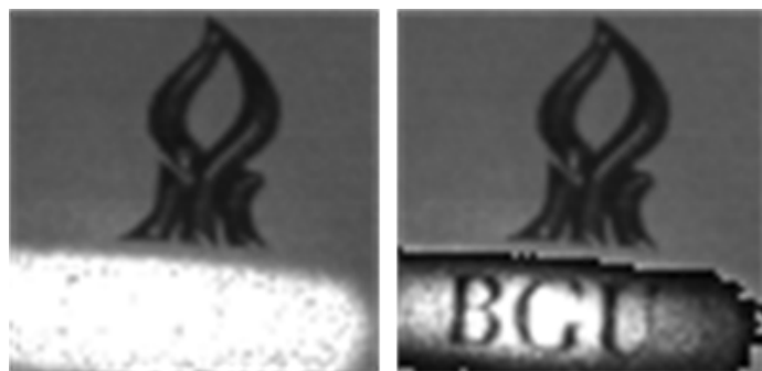
Figure 2. (a) Scene observed with a traditional CMOS APS sensor. (b) Scene observed with our in-pixel auto exposure CMOS APS sensor
